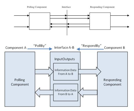
Interface has two sets of inputs and outputs. Each set is defined by the direction of the communication flow between the Components.
